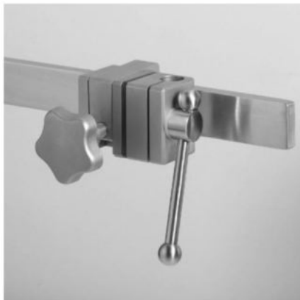
24-799-02 Clamp socket made of stainless steel, for height-adjustable stand Ø 16 mm, electrically insulated up to 1.5 kV AC, holding width of 35 mm for rails 25/32 x 8/12 mm.
