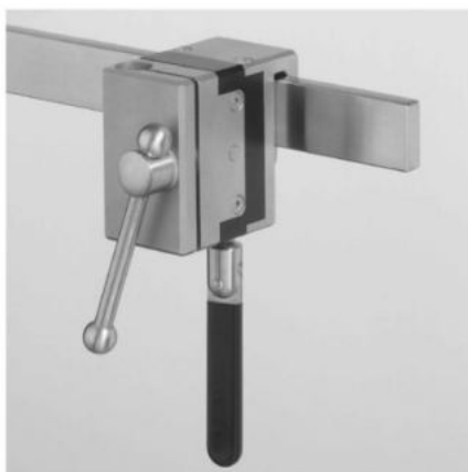
24-799-05 Clamp socket made of stainless steel, for height-adjustable stand Ø 16 mm, electrically insulated up to 4.5 kV AC, holding width of 50 mm for rails 25/32 x 8/12 mm.
