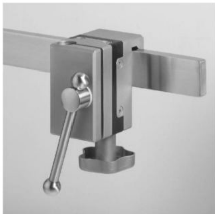
24-799-01 Clamp socket made of stainless steel, for height-adjustable stand Ø 16 mm, electrically insulated up to 1.5 kV AC, holding width of 35 mm for rails 25/32 x 8/12 mm.
