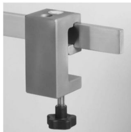
24-799-06 Clamp socket made of light metal, holding width 50 mm, for screw stand Ø 16 mm/M10, for rails 25/35 x 8/10 and tubes Ø 12 - 35 mm.
