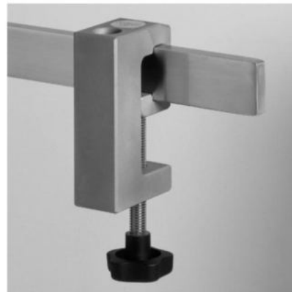
24-799-03 Clamp socket made of light metal, holding width 35 mm, for screw stand Ø 16 mm/M10, for rails 25/35 x 8/10 and tubes Ø 12 - 35 mm.
