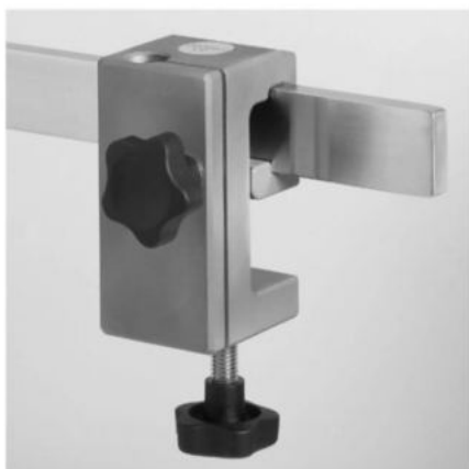
24-799-04 Clamp socket made of light metal, holding width 50 mm, for height-adjustable stand Ø 16 mm, for rails 25/35 x 8/10 and tubes Ø 12 - 35 mm.
